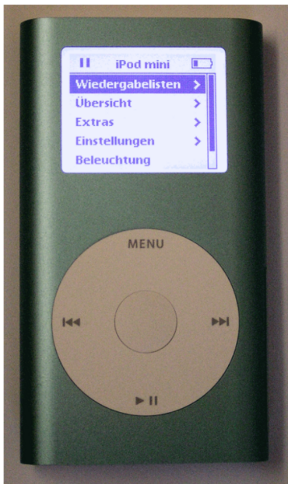
Colored iPod Mini cases are dyed following anodizing and before thermal sealing
