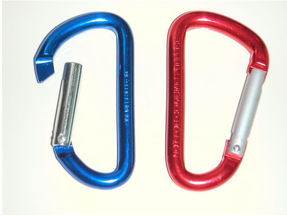
These carabiners have an anodized aluminium surface that has been dyed; they are made in many colors.
