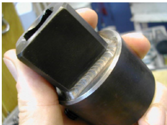
GTAW fillet weld
