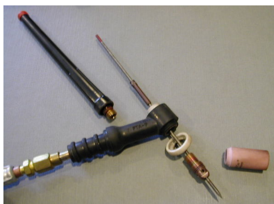
GTAW torch, disassembled
