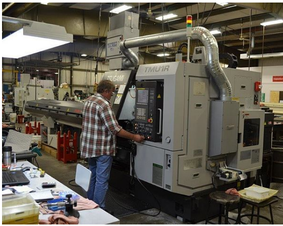
A Tsugami multifunction turn mill machine used for short runs of complex parts.
