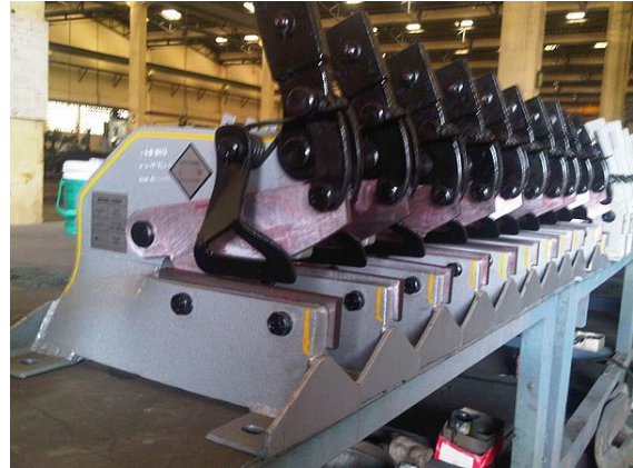
Shearing machine can cut flat bar up to 6mm.
