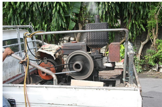
A diesel powered welding generator (the electric generator is on the left) as used in Indonesia.
