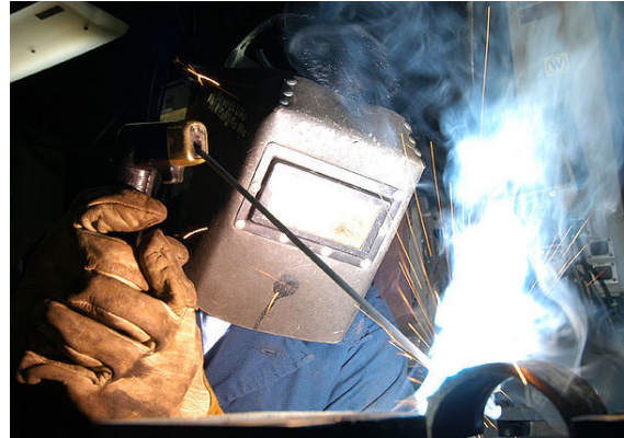
Shielded metal arc welding
