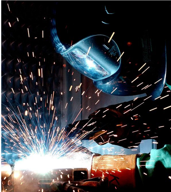
Gas metal arc welding
